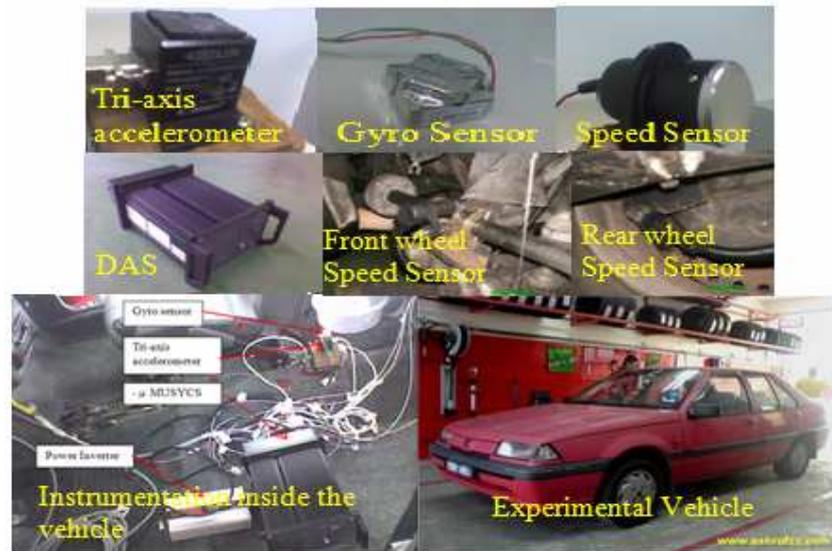
Figure 7: In-vehicle instrumentations
