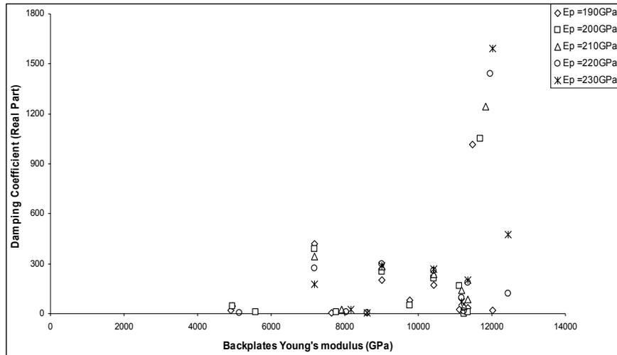
Figure 9a: Variation of the damping coefficient with frequency for different young's modulus of the back plates of the pads.
