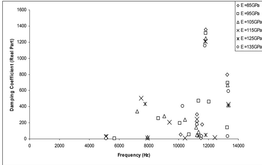
Figure 8a: Variation of the damping coefficient with frequency for different Young's modulus of the disc.
