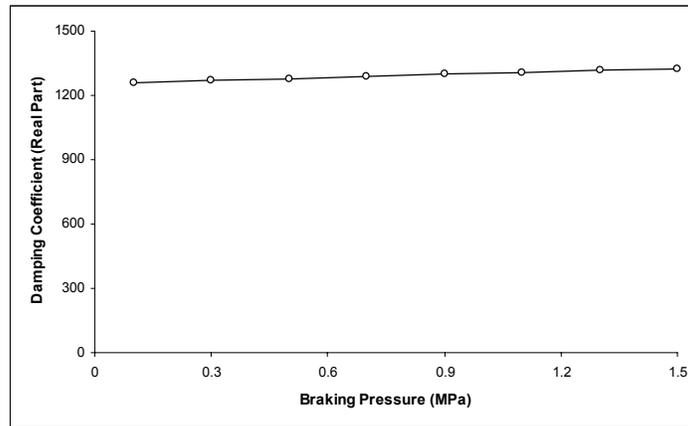
Figure 7b: Variation of the damping coefficient with braking pressure at frequency 12 kHz.
