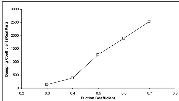
Figure 6b: Variation of the damping coefficient with friction coefficient at frequency 12 kHz.
