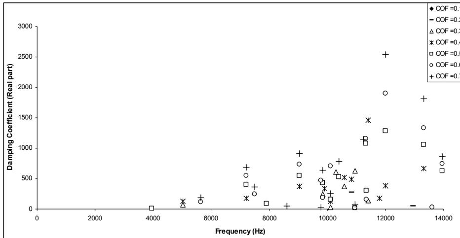
Figure 6a: Unstable modes with friction coefficient varied from 0.1 to 0.7.
