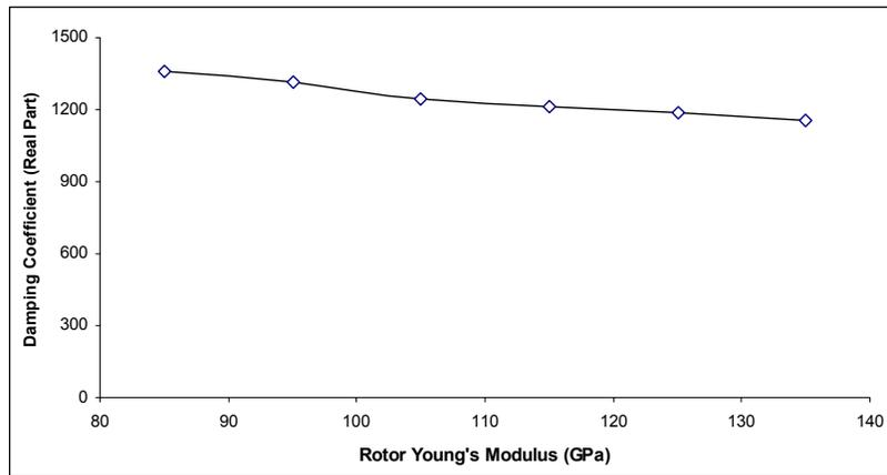
Figure 8b: Variation of the damping coefficient with young's modulus of the disc at frequency 12 kHz
