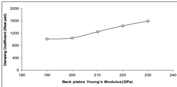
Figure 9b: Variation of the damping coefficient with young's modulus of the back plates of the pads at frequency 12 kHz.
