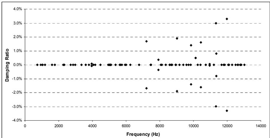
Figure 3: Damping ratio vs. frequency for the disc brake model
