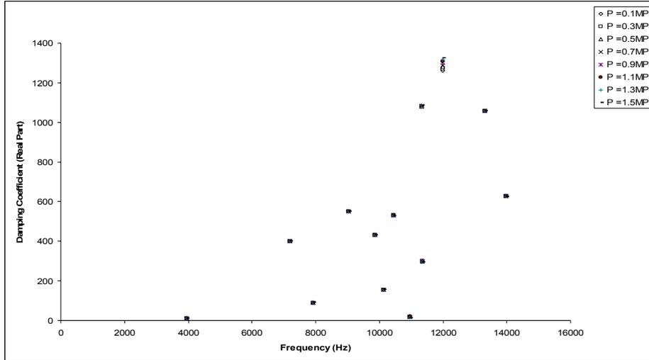
Figure 7a: Unstable modes with braking pressure varied from 0.1 to 1.5 MPa.
