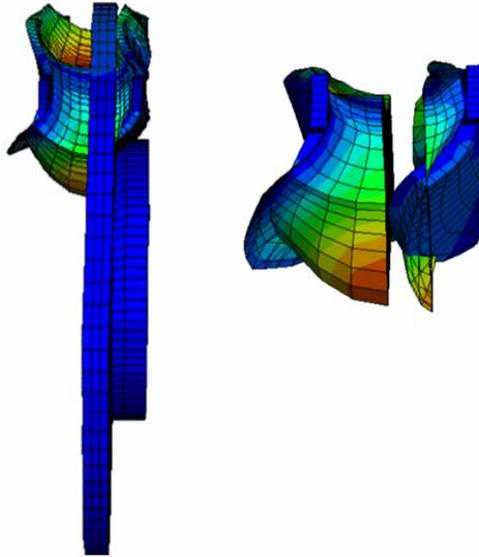
Figure 4: Vibration mode of the disc brake model at 12 kHz.
