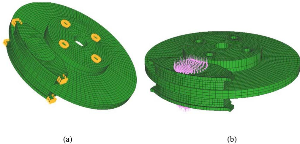
Figure 1: The simplified disc brake model
