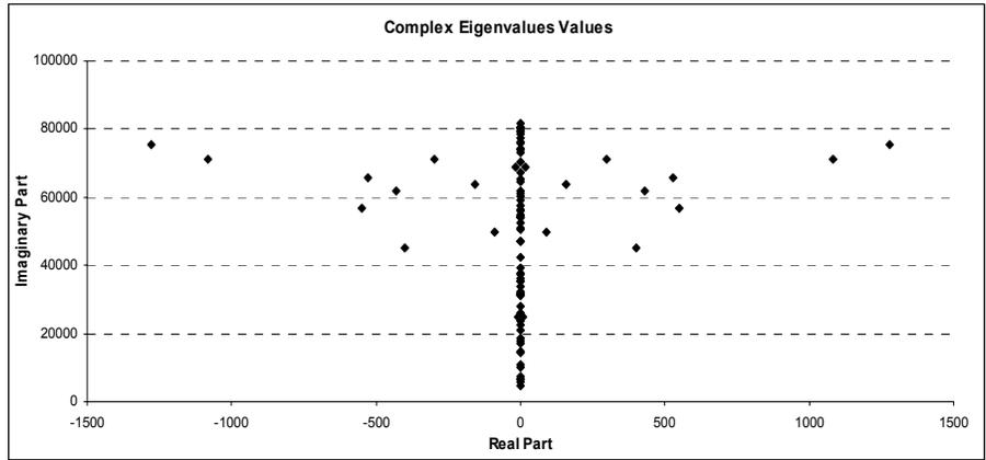
Figure 2: Eigenvalues extracted from the disc brake model plotted on the complex plane.
