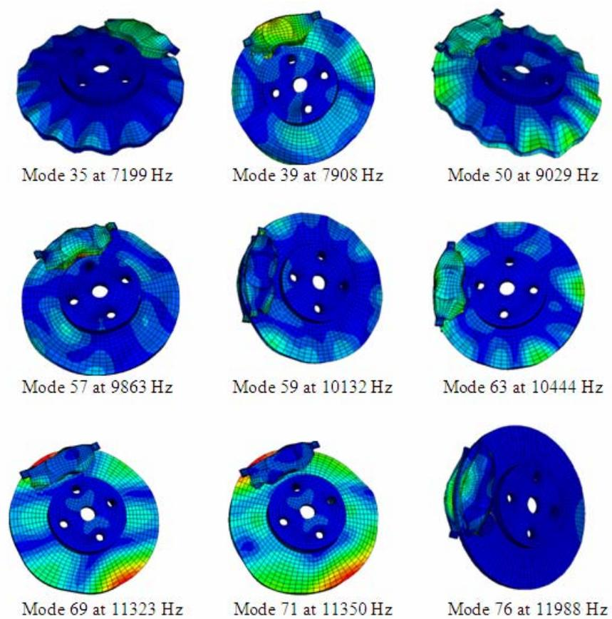
Figure 5: Example of unstable modes of the disc brake model.
