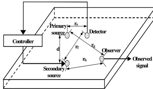
Figure 1: Schematic diagram of the AVC structure
