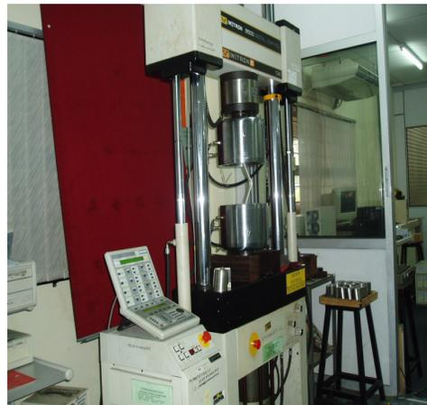
Figure 4: The test set-up for the compression test
