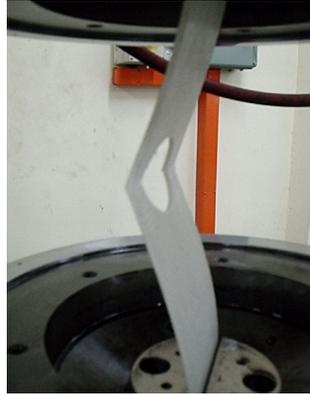
Figure 5: Buckled shape of panels with cut-outs
