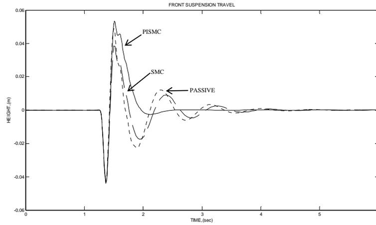
Figure 2: Front suspension travel
