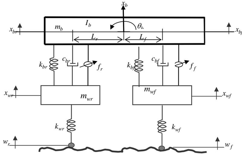
Figure 1: The active suspension for the half car model
