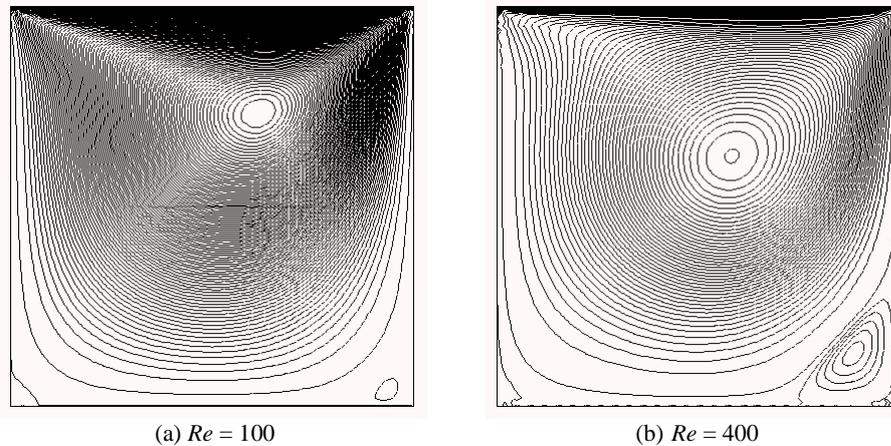
Figure 1: Streamline plots for two values of Reynolds numbers.
