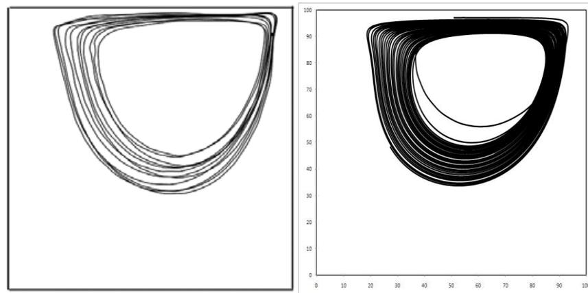
Figure 3: Orbits of particle plotted from experimental investigation of Tsorng *et.al* [1] (left) and current method (right).
