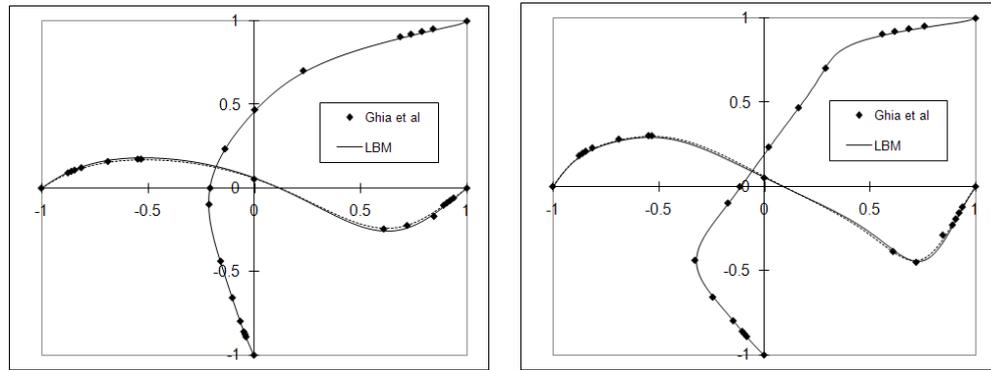
Figure 2: Comparisons of velocity profiles between LBM and benchmark results for  $Re = 100$ (left) and  $Re = 400$  (right).
