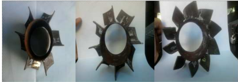
Figure 14 : Swirlers with 6, 8 and 10 vane blades
