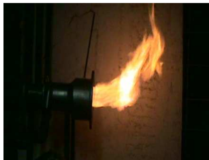
Figure 1: Gas burner flame with yellow-red color domination
