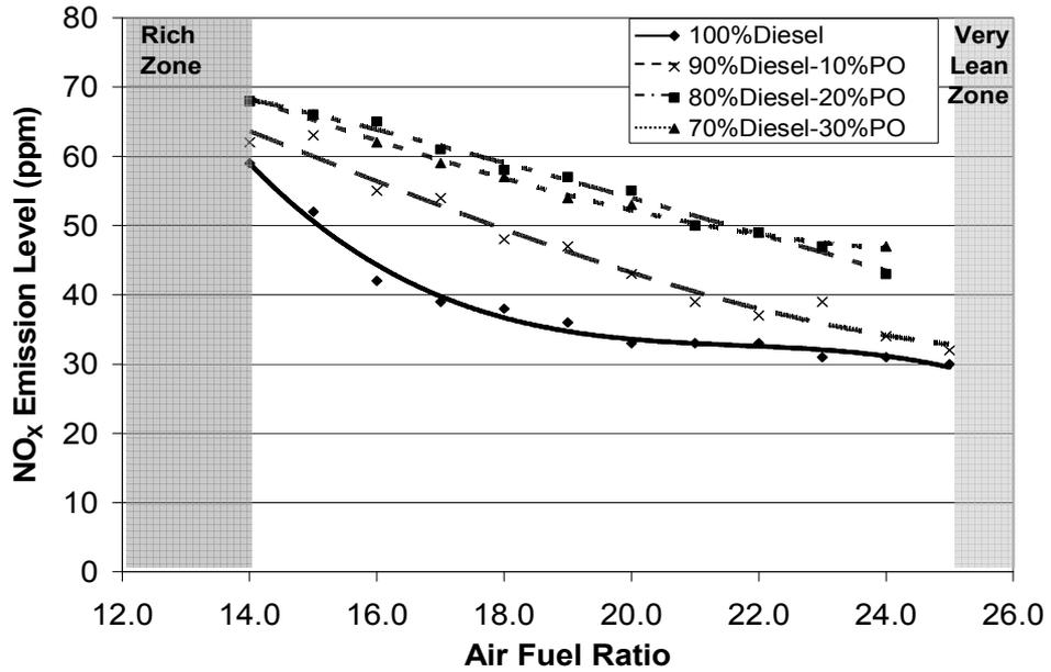
Figure 6 : NO<sub>x</sub> emissions of the combustions of various blended fuels at 5kg/h
