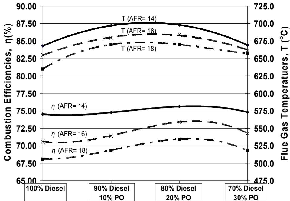
Figure 8: Combustion efficiencies of various blended fuels at different air fuel ratio
