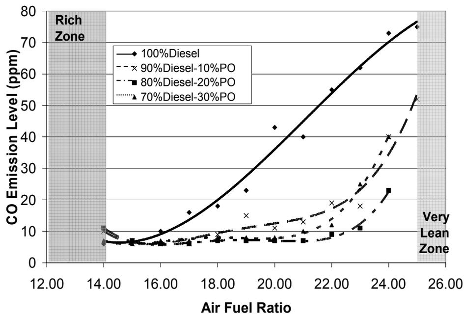
Figure 5 : CO emissions of the combustions of various blended fuels at 5kg/h
