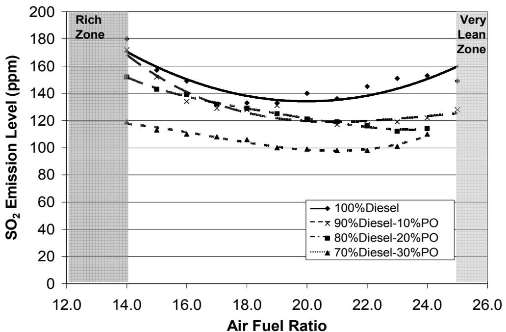
Figure 7: SO<sub>2</sub> emissions of the combustions of various blended fuels at 5kg/h
