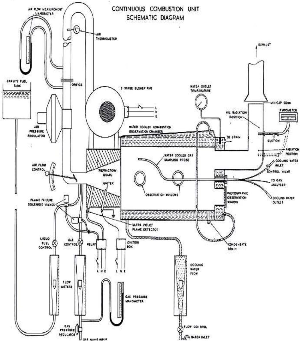
Figure 2 : Schematic diagram of a continuous spray combustion unit with water-cooled furnace (Hilton and Hewett, 1980).
