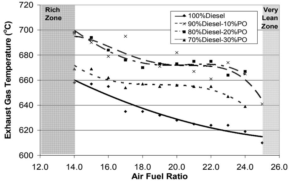
Figure 3: Exhaust Temperatures of the combustions of various blended fuels a 5kg/h
