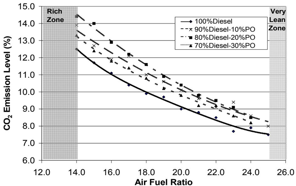
Figure 4: CO<sub>2</sub> emissions of the combustions of various blended fuels at 5kg/h
