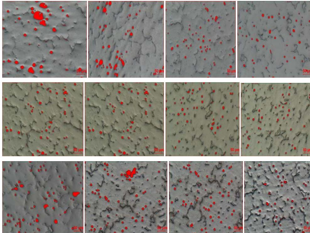
Figure 9: Porosity fraction measurements at 780°C
