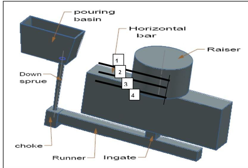
Figure 1 : Mould with downsprue, raiser, ingate and cavity bar with bottom filling gating system.
