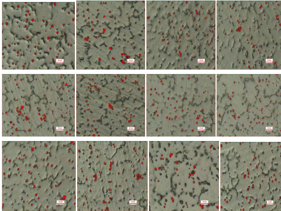
Figure 7: Porosity fraction measurements at 680°C
