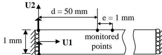
Figure 3: Plate under extension in explicit step, excited with anti-symmetrical mode,  $A_0$
