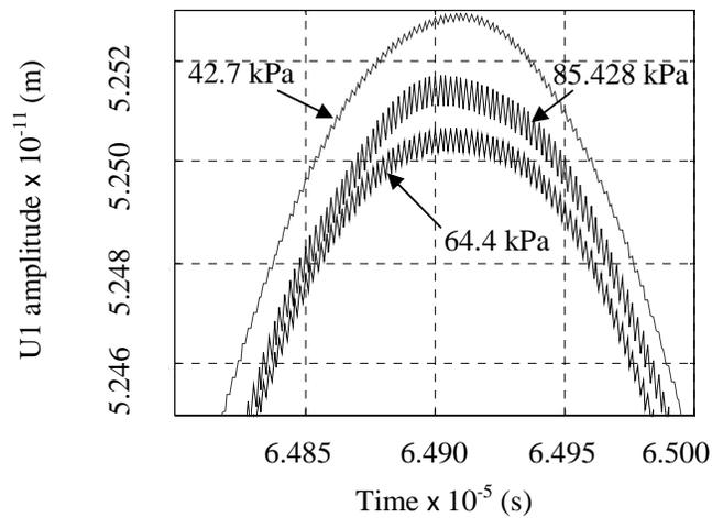
Figure 9 : Zoom views of U1 amplitude peaks in time domain for plate under bending (load pattern as in Figure 5) with various strain values at d=50mm.
