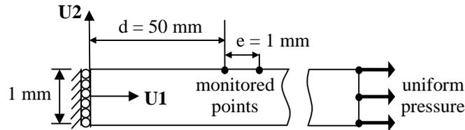
Figure 2: Plate under extension in static step with uniform pressure pulling outward to simulate the uni-axial loading.
