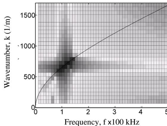
Figure 1: Overlapping of dispersion curve provided by SAFE (straight line) and ABAQUS
