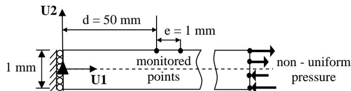
Figure 4: Plate under bending in static step with asymmetrical pressure applied.
