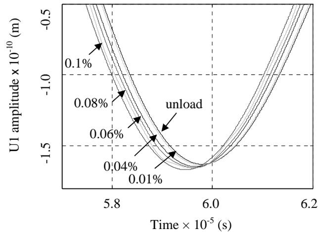
Figure 7 : Zoom views of U1 amplitude peaks in time domain for plate under no load and plate under uni-axial (extension) load with various strain values at  $d=50\text{mm}$ .
