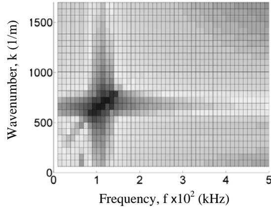
Figure 10 : A mode Dispersion curve of wavenumber,  $k$  (1/m) versus Frequency,  $f$  (kHz) for plate under extensional with 0.1% strain (70MPa)
