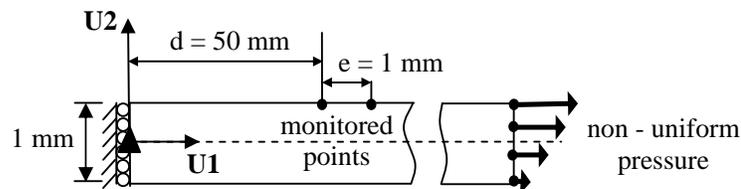
Figure 5: Plate under bending in static step with asymmetrical pressure applied.
