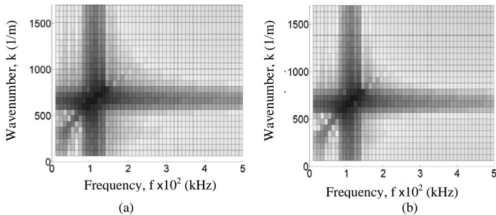
Figure 11 : Antisymmetrical mode dispersion curve of wavenumber,  $k$  (1/m) versus frequency,  $f$  (kHz) for plate under bending (a) pattern in Figure 4 with 1.08MPa (0.00154% strain) and (b) load pattern as in Figure 5 with 85.428 kPa (0.000122% strain)
