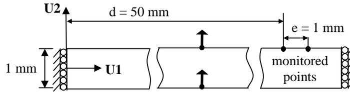
Figure 6: Plate under bending in explicit step, excited with anti-symmetrical mode,  $A_0$
