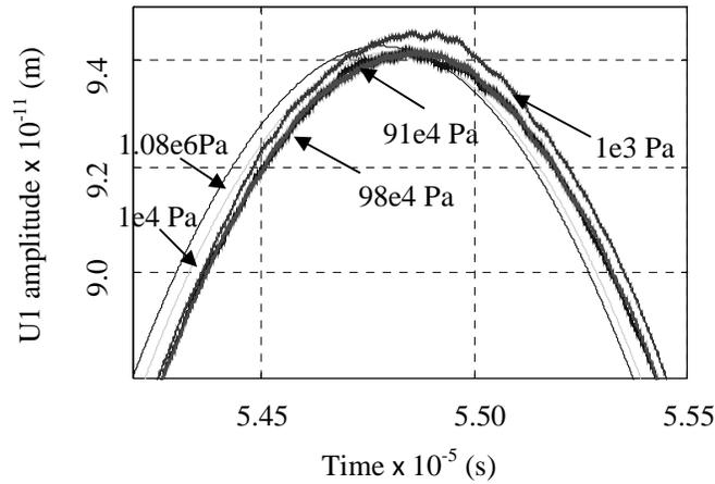
Figure 8 : Zoom views of U1 amplitude peaks in time domain for plate under bending (load pattern as in Figure 4) with various strain values at d=50mm.
