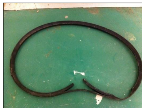
Figure 10 Picture of the broken belt.
