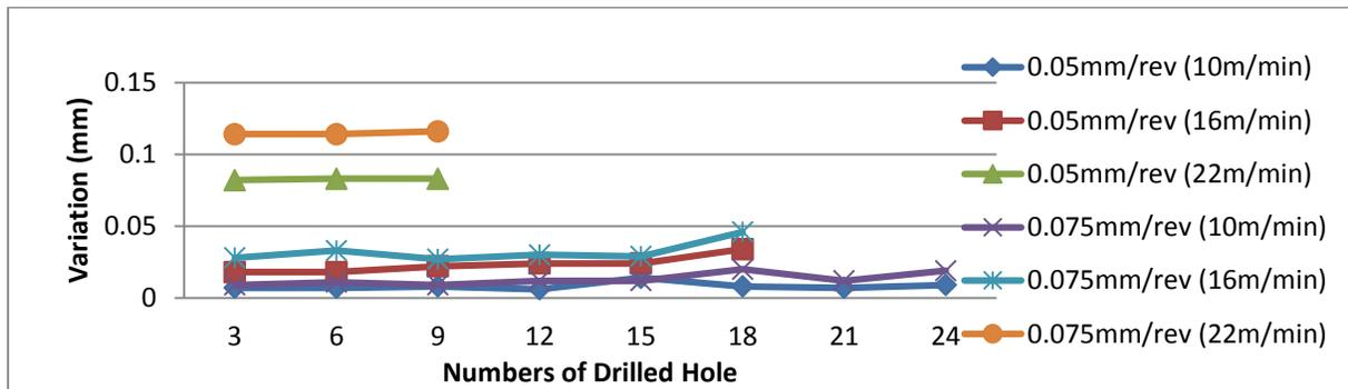
Figure 4a: Dimensional Accuracy for Tool A (Coolant)
