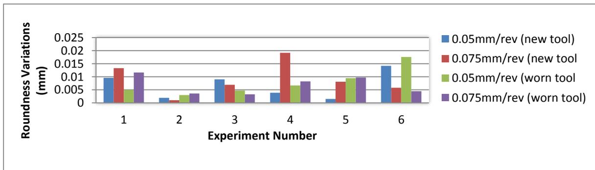
Figure 5c: Roundness of Drilled Holes for New and Worn tool.
