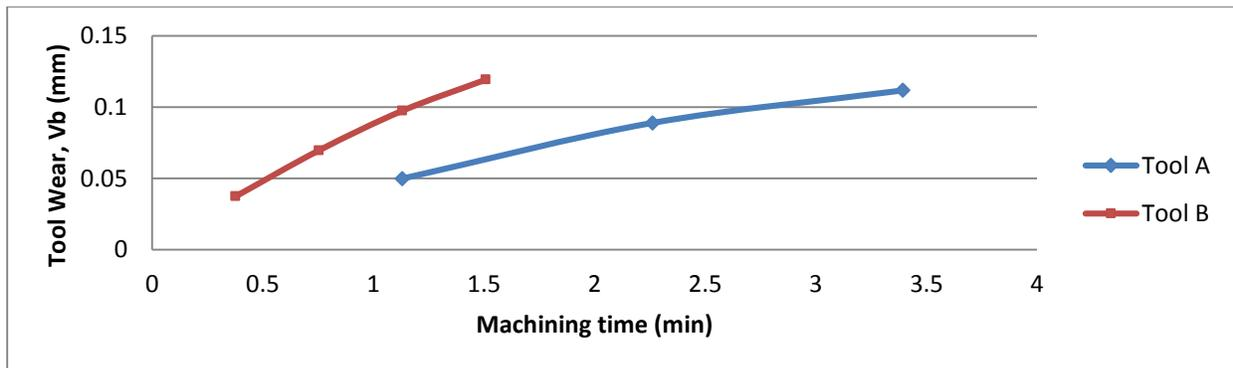
Figure 1c: Tool Wear of Tool A and Tool B at 22 m/min Cutting Speed.
