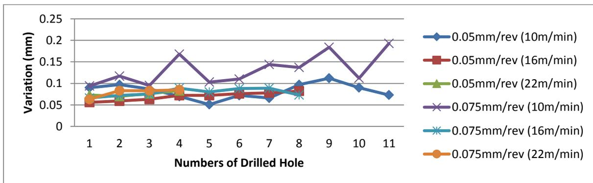
Figure 4b: Dimensional Accuracy for Tool B (No Coolant)
