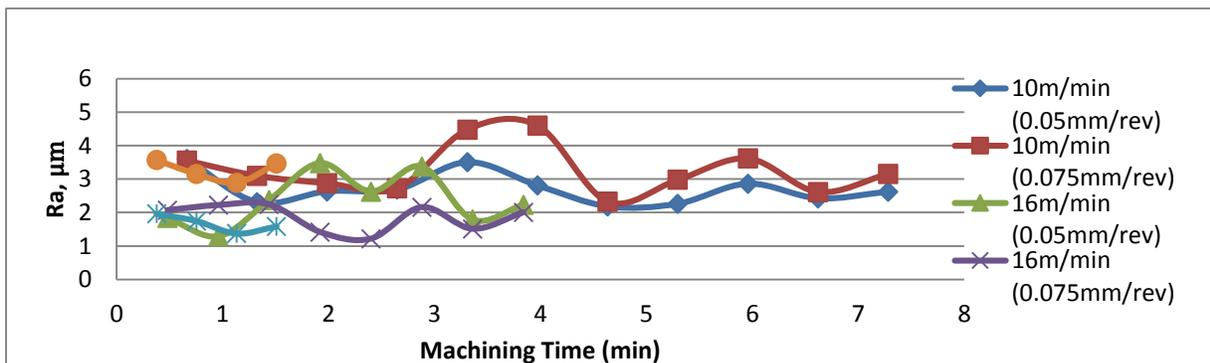
Figure 3b: Surface Roughness for Tool B at various cutting speed
