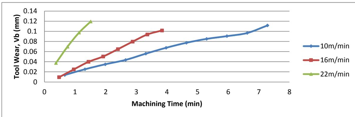
Figure 1e: Comparison of Tool Wear of Tool B at various Cutting Speed.
