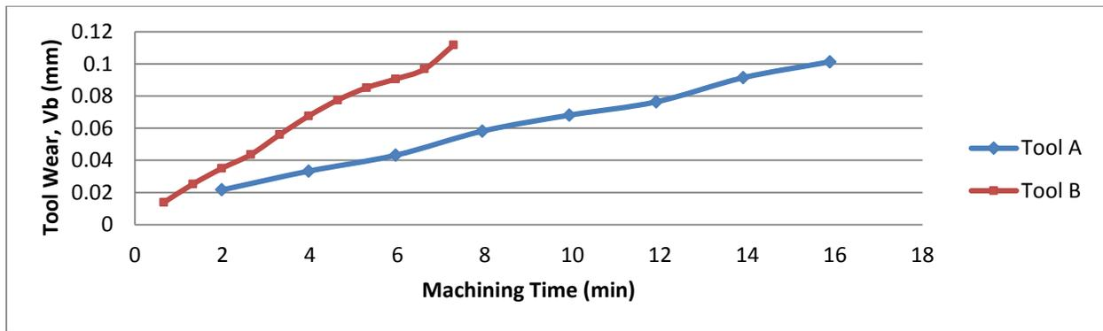
Figure 1a: Tool Wear of Tool A and Tool B at 10 m/min Cutting Speed.
