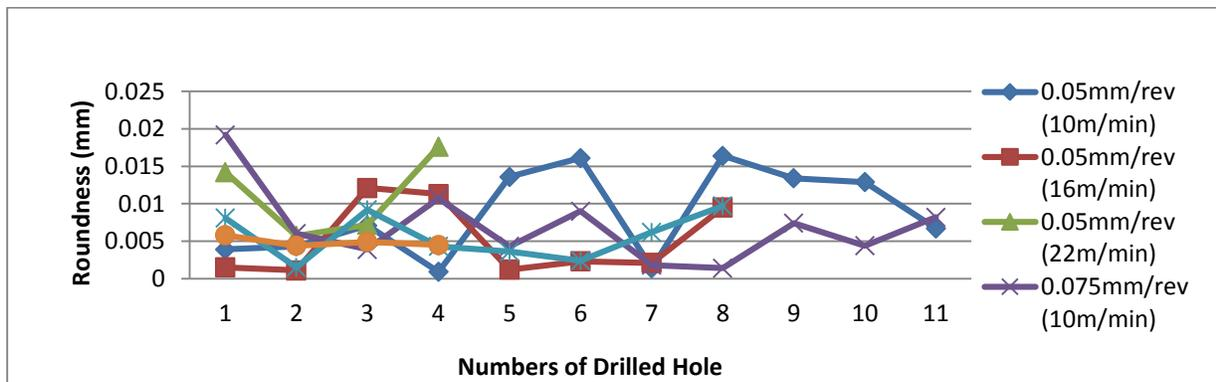
Figure 5b: Roundness of Drilled Holes for Tool B (No Coolant).
