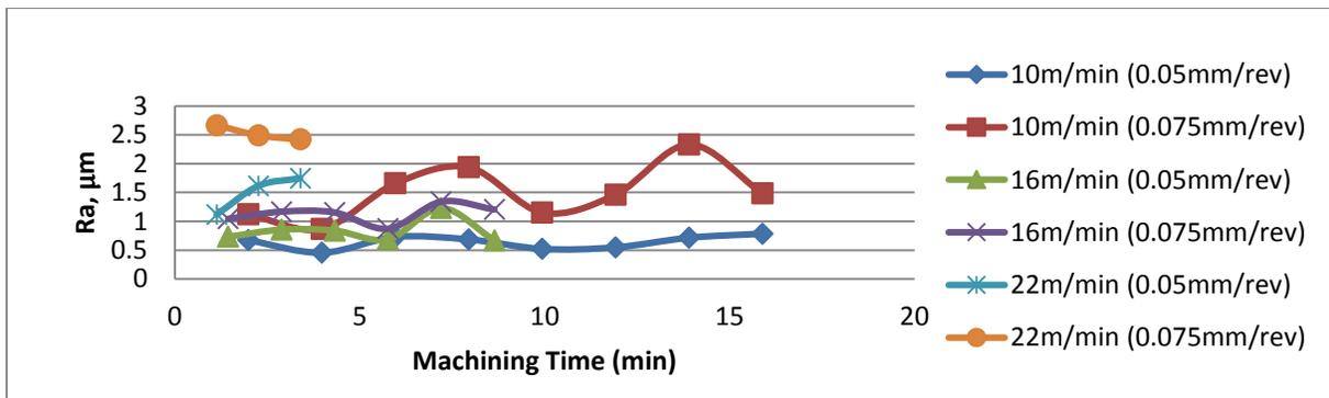
Figure 3a: Surface Roughness for Tool A at various cutting speed
