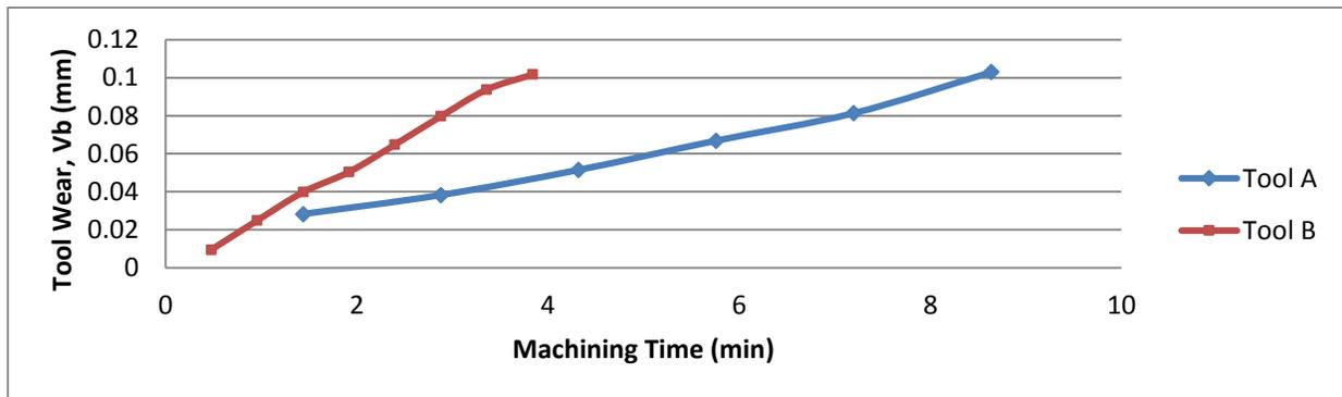
Figure 1b: Tool Wear of Tool A and Tool B at 16 m/min Cutting Speed.
