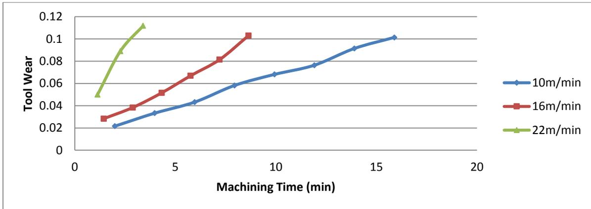
Figure 1d: Comparison of Tool Wear of Tool A at various Cutting Speed.
