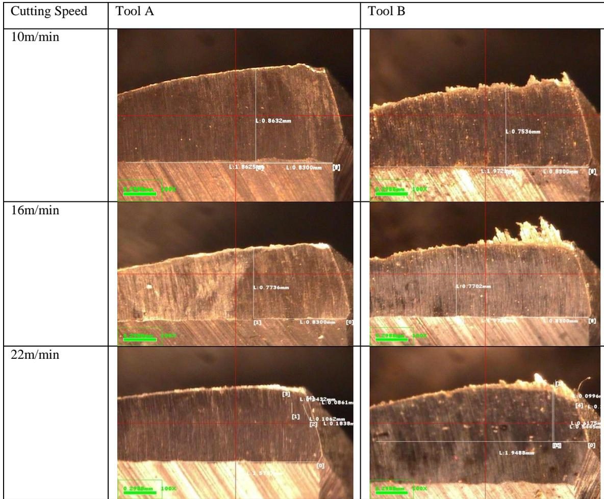
Figure 2: Image of worn tools at initial drilling stage
