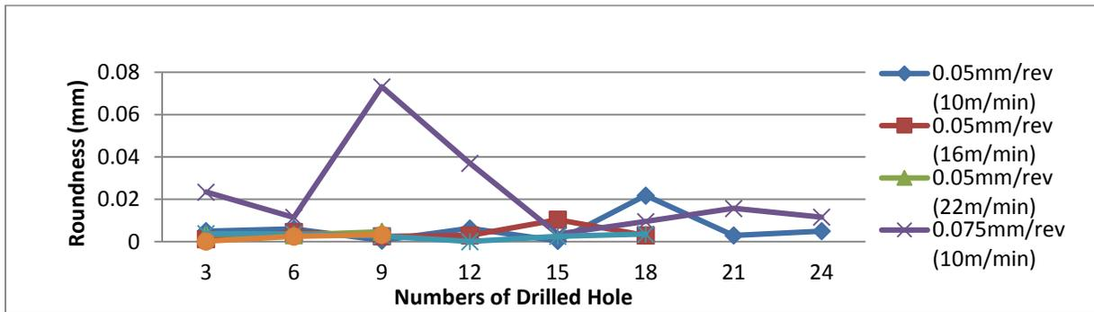
Figure 5a: Roundness of Drilled Holes for Tool A (Coolant).
