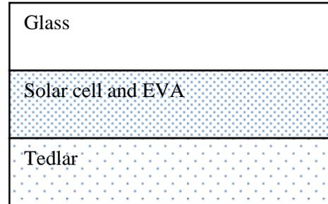
Figure 2: Cross section of the PV
