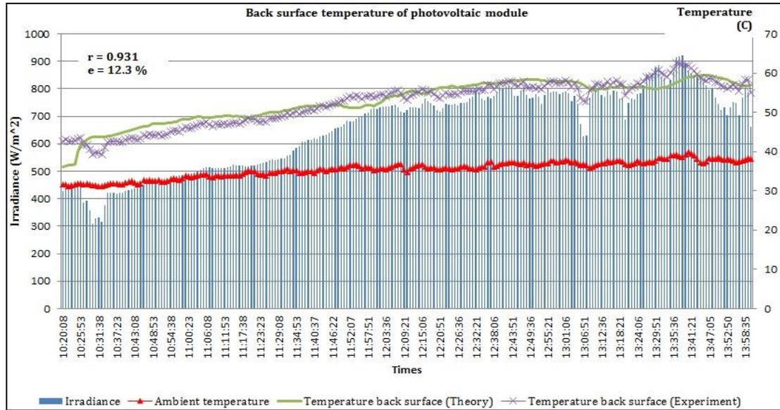
Figure 4: The back surface temperature of photovoltaic (no sudden fluctuation)
