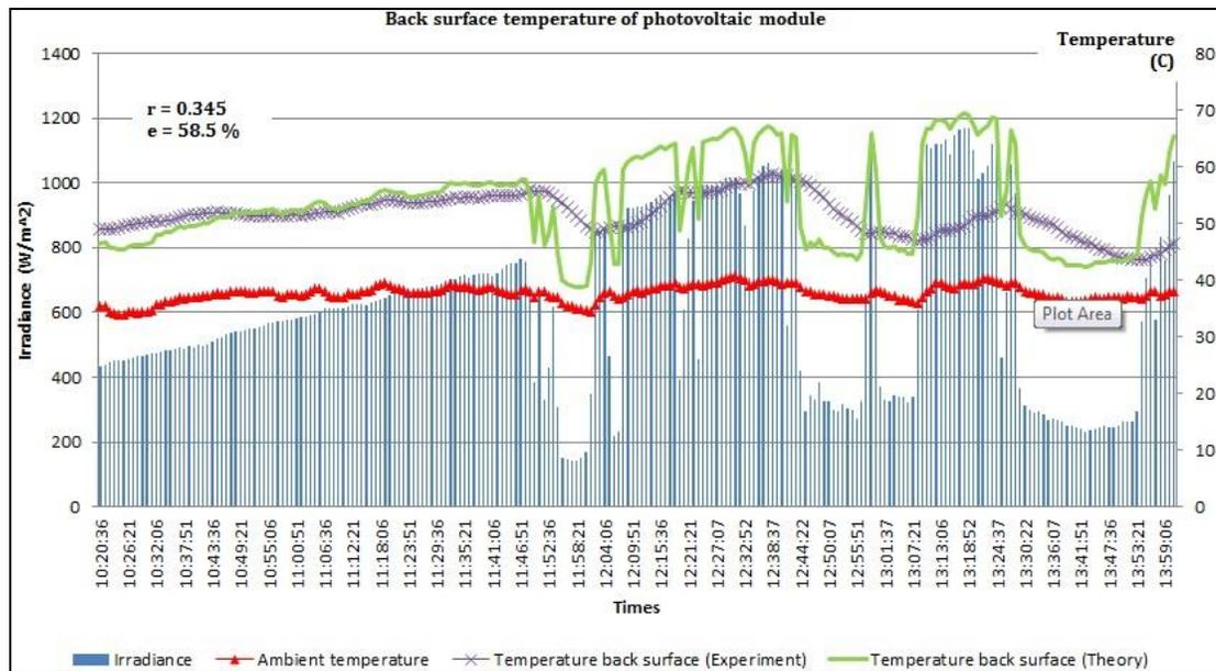
Figure 5: The back surface temperature of photovoltaic (sudden fluctuation)
