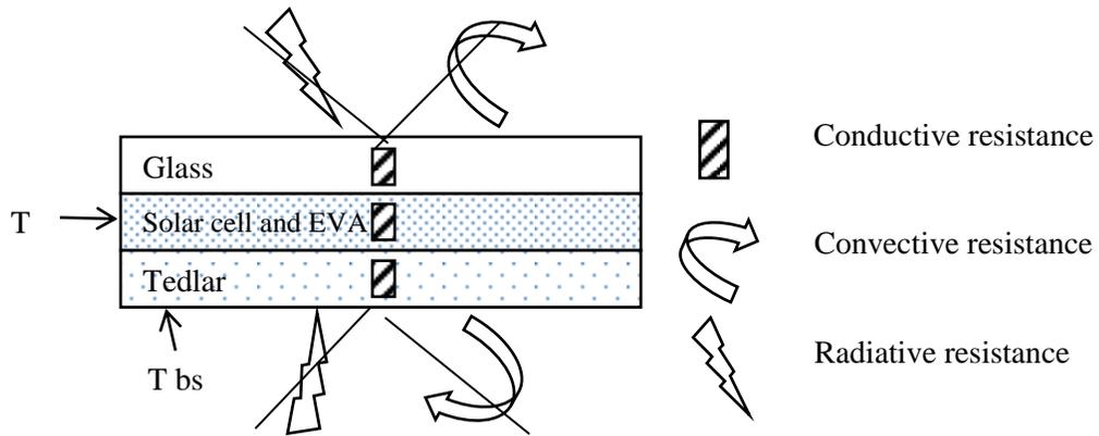
Figure 3: Heat transfer for the PV
