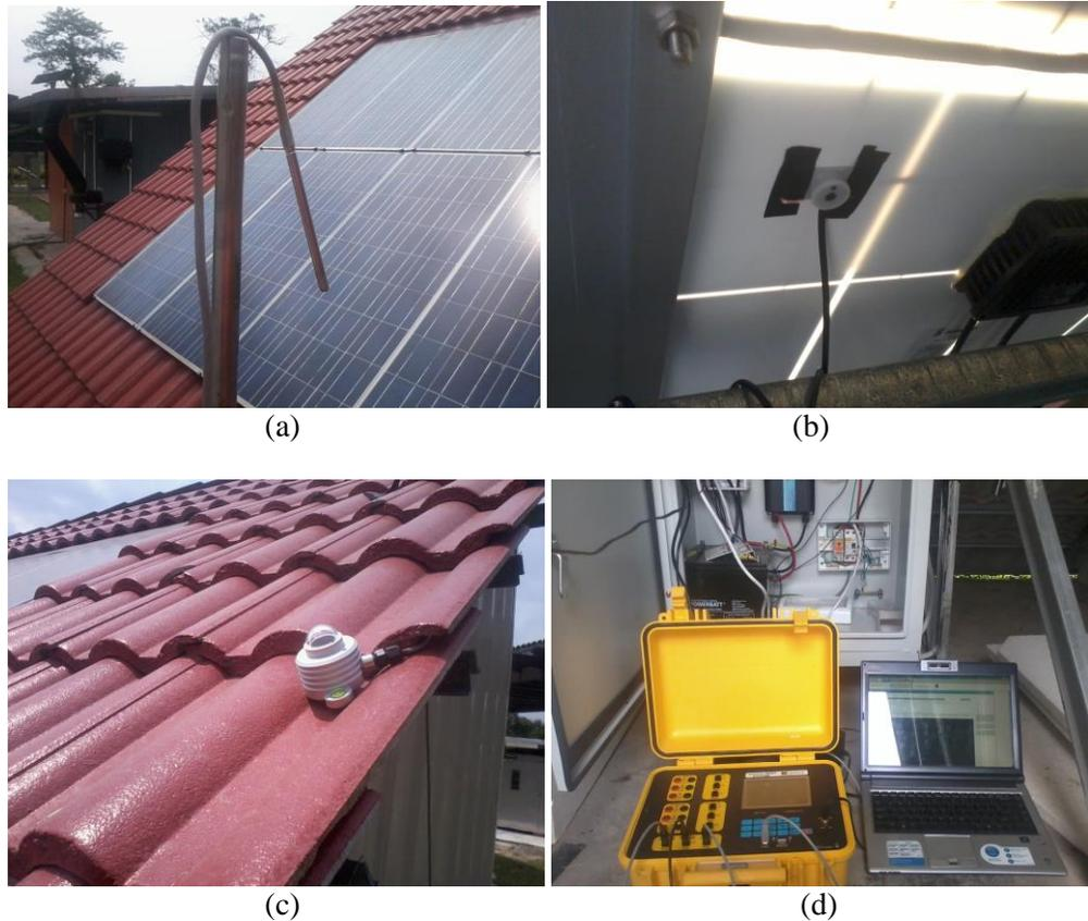
Figure 4 (a): Measuring ambient temperature, (b) Measuring back surface temperature, (c) Measuring the irradiance, (d) Data logger system
