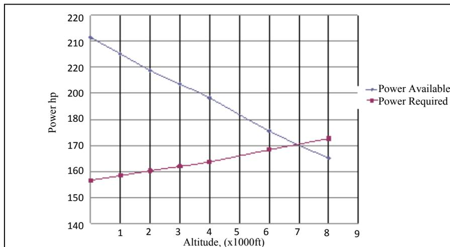
Figure 4: Power Required For Hovering Versus Altitude
